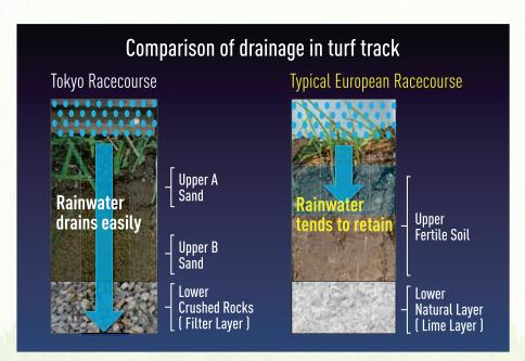
To cope with Japanese frequent rainfall, the base of the turf track is composed of sandy soil for the upper layer and crushed rocks for the lower layer, both of which have high drainage properties. Therefore, after rainfall it is less likely to become too soft and the track can be kept relatively level.
