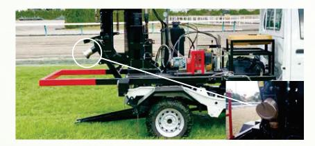
This special vehicle (left) has been developed by the JRA and has been in use since 1989. It can measure turf hardness over the whole of the track by dropping a horseshoe-shaped 6kg weight with an accelerometer every 10 meters.
