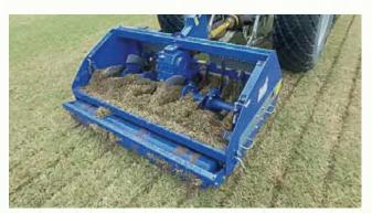
In recent times, aeration of the turf track has been carried out by machines such as the Verti Drain and Shock Waves in order to add more cushioning to the turf.
